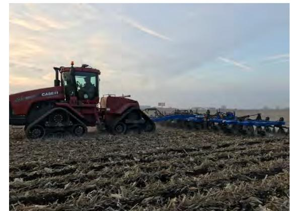
Figure 3. Case IH Steiger® Series with Strip-Till Bar
